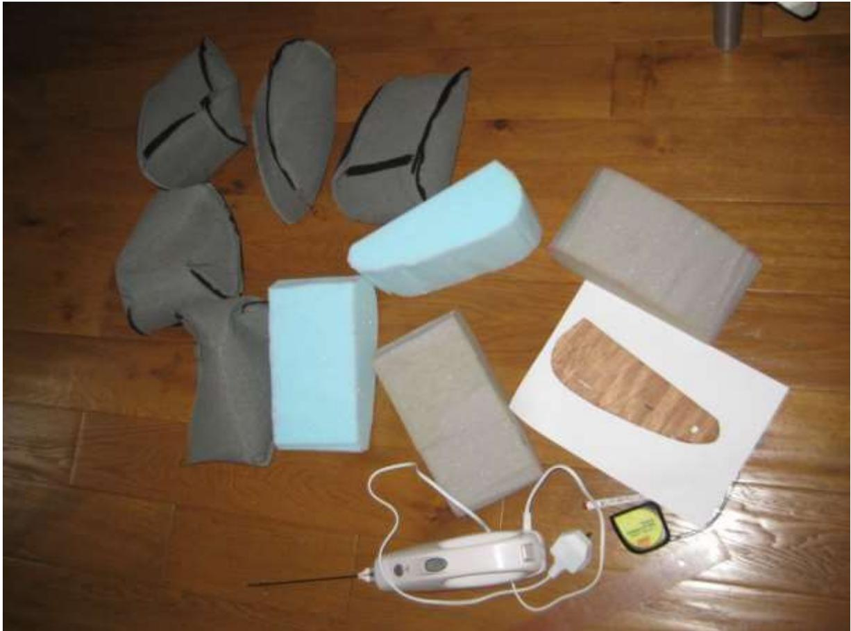
Note; the covers are inside out ready to be to be stuffed with the two types of foam shown here; Softer, HR40, and harder foam.
